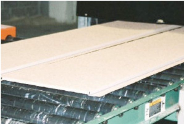
Stucco Panels exiting bake oven
